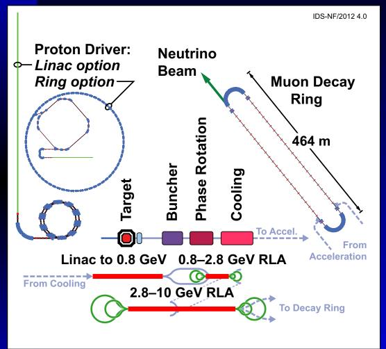
10 GeV muon energy 1E21 useful muon decays per straight and polarity, in 1E7 s
