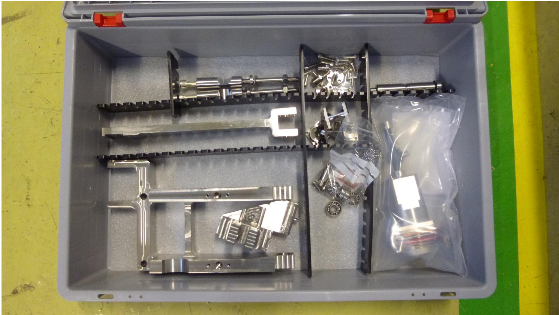
Tuner mechanics, after disassembly, and motor
