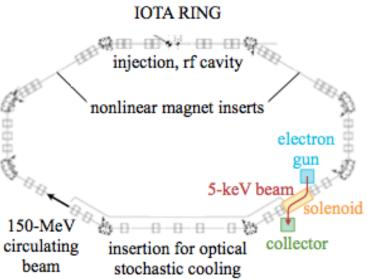
Two options for an integrable nonlinear optic using an electron lens:
