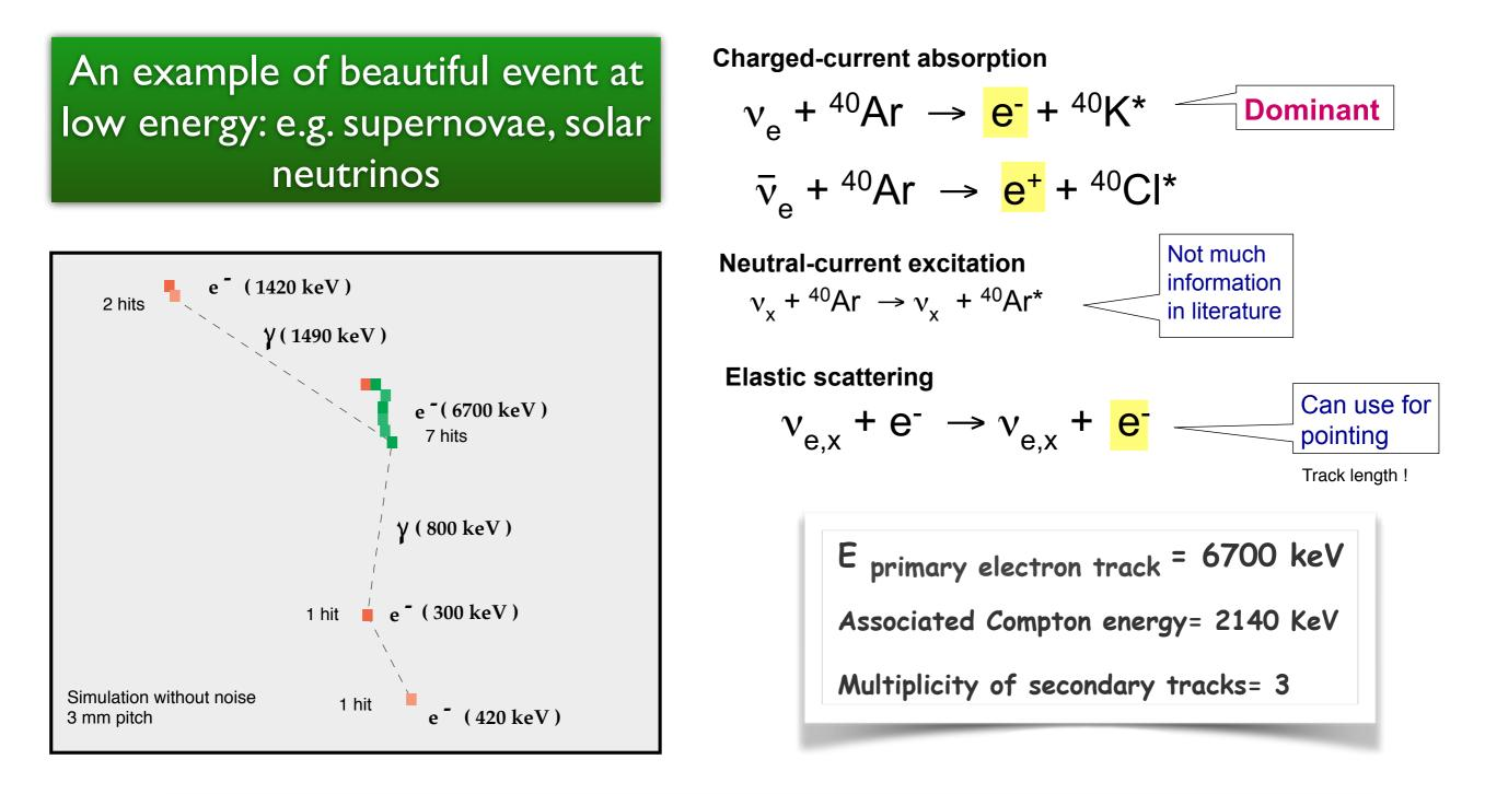
100 keV hit (i.e. S/N > 100 for mip) and 3mm wire pitch needed !
