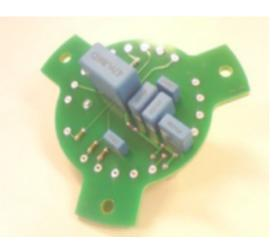
✓ PMT ordered and bases are fabricated at KEK following design from ArDM.
