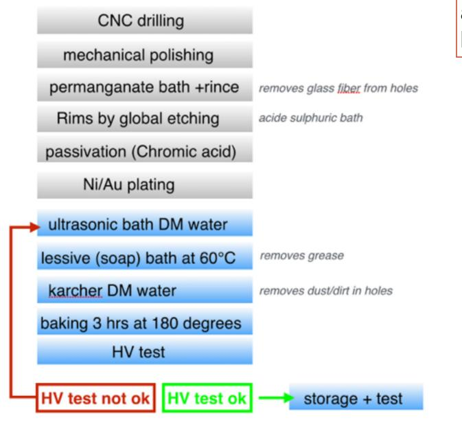
LEM cleaned then powered in controlled atmosphere to check spark threshold + leakage current.
