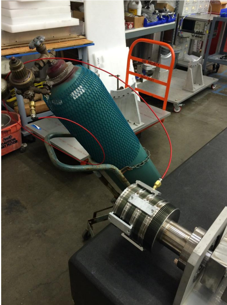
Figure 2: MICE actuator hooked up to argon tank for functional test
