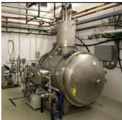
Spoke Test Cryostat (STC)
