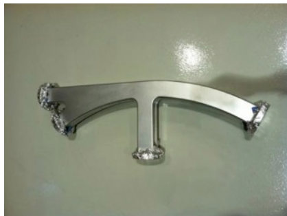
Vacuum chambers for dipoles (received)
