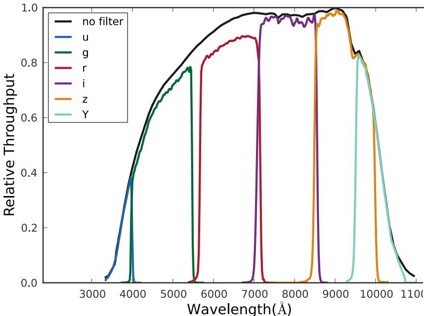
System throughput vs wavelength is measured by DECal, is monitored through periodic scans with some attention to the blue and red filter edges. Data product of the average response is provided.
