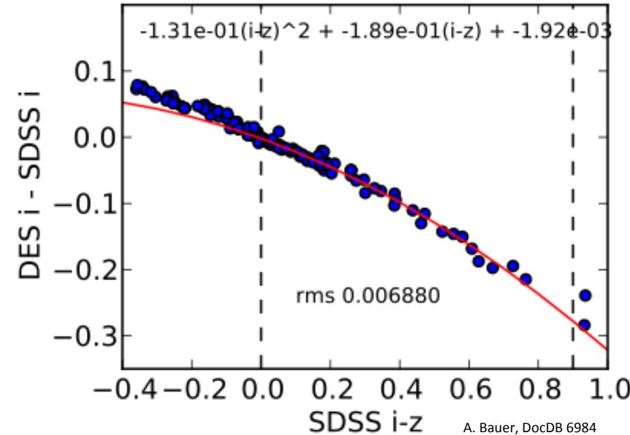
Transfer functions derived from the system response maps to determine the DES to SDSS transformation in magnitudes and color for a catalog of stellar spectral types.
