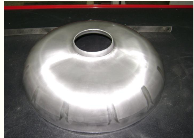
Beginning of forming trials with aluminum
