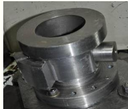
High RRR end group Machining in progress
