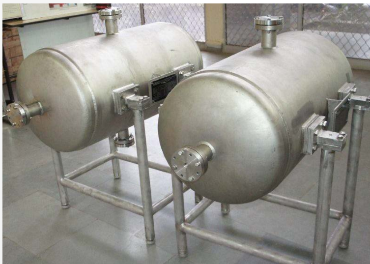
Titanium vessels fabricated at M/s TITAN, Chennai
