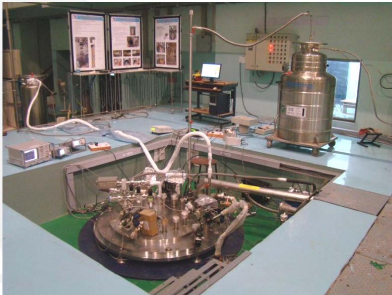
Transfer of liquid helium in the VTS cryostat
