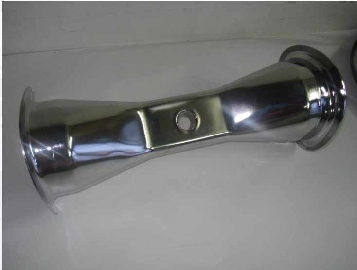
Spoke assembly after electropolishing.
