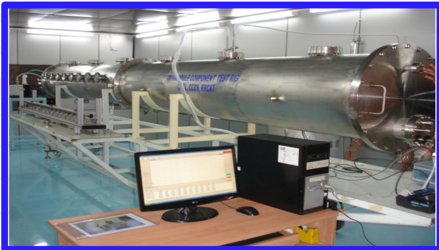
Cryomodule component test rig
