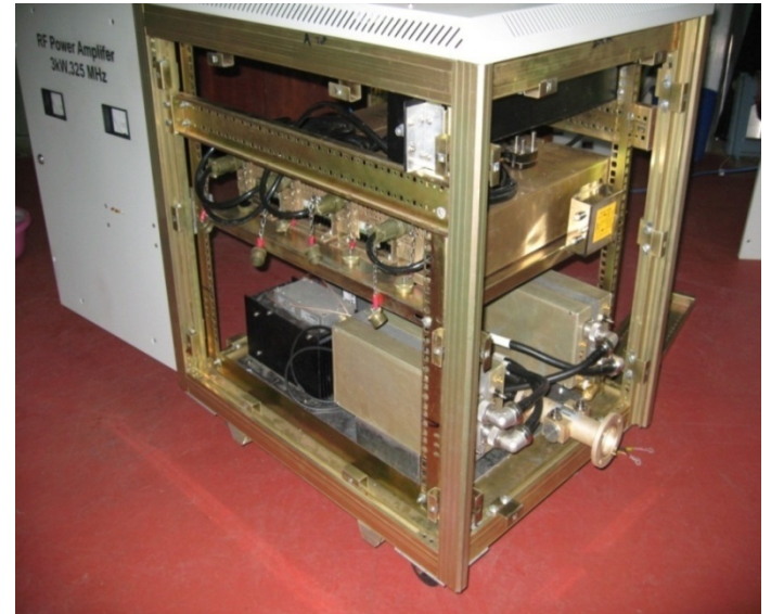
Fully assembled 3 kW whole Unit
