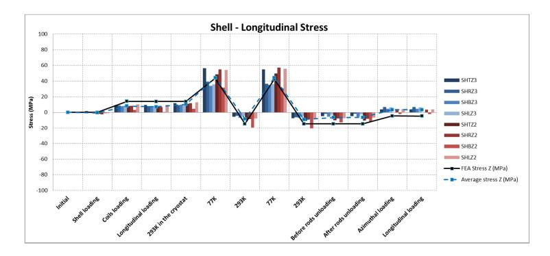
Path dependent effects introduced by friction Numerical analysis performed with multiple sub-steps Fine-tuning of the friction coefficient (from 0.2 to 0.3)
