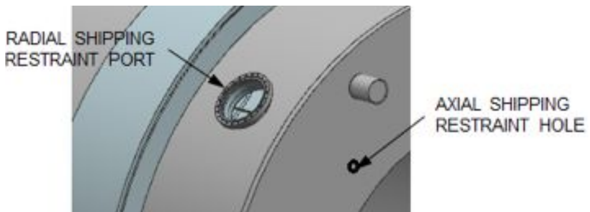
Figure 6.21. PS axial and radial shipping restraints.
