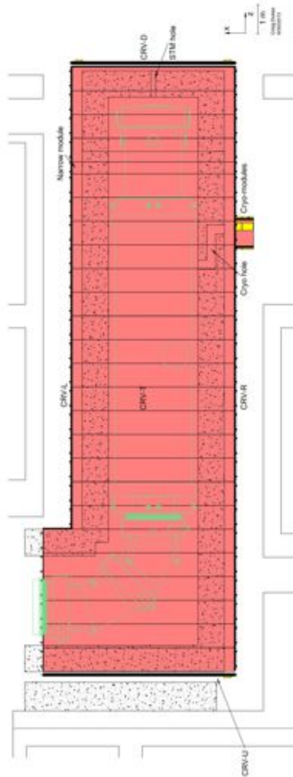
Figure 10.16. Plan view of the CRV showing the outlines of the shielding and TS and DS. The module supports are not shown. Front-end board enclosures are shown in yellow.
