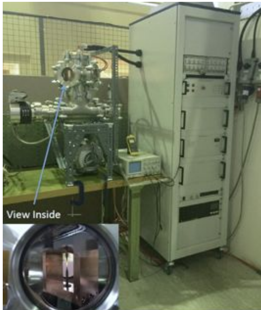
Figure 4.159. Vacuum test rig, with shaped tungsten test piece installed for pulsed current tests.
