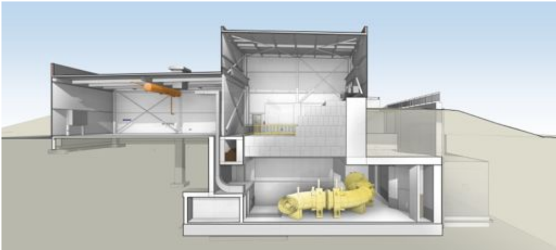
Figure 5.6 A transverse section of the detector hall showing the layout of the Transport Solenoid.
