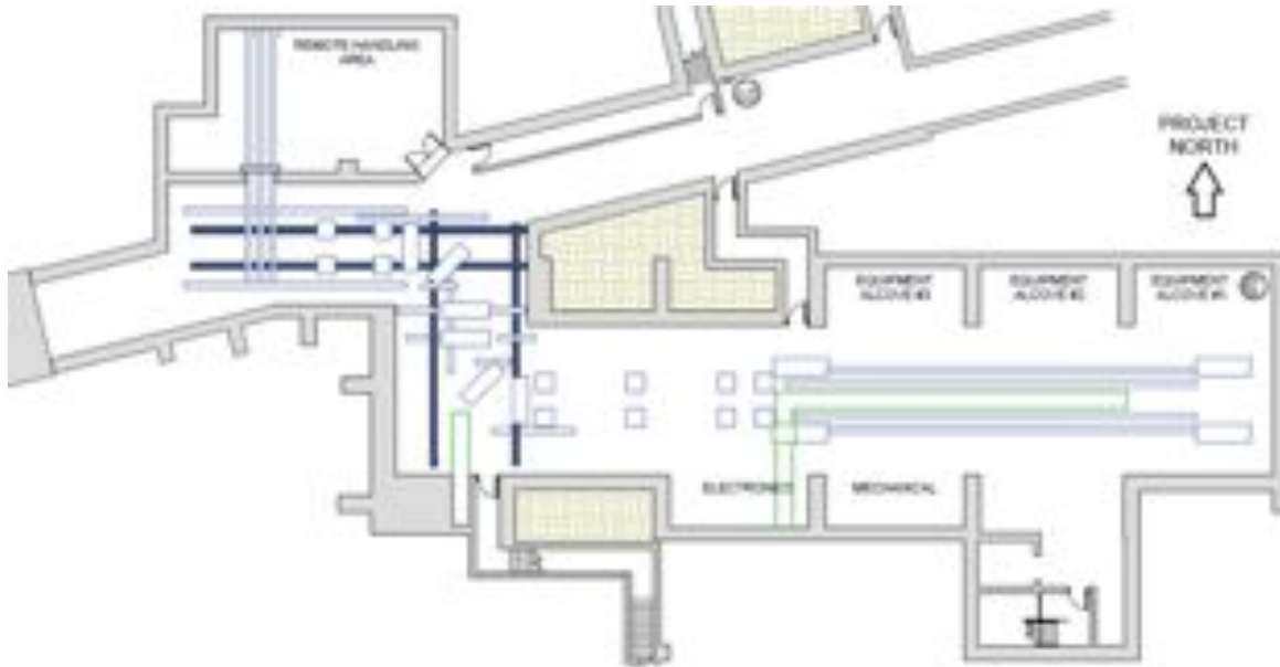
Figure 6.121. Layout of the Mu2e floor track system.
