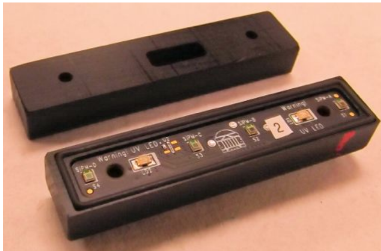
Figure 10.21. The counter manifold cover top (above) and bottom (below). The O-ring and counter motherboard with its SiPMs and flasher LEDs can be seen.
