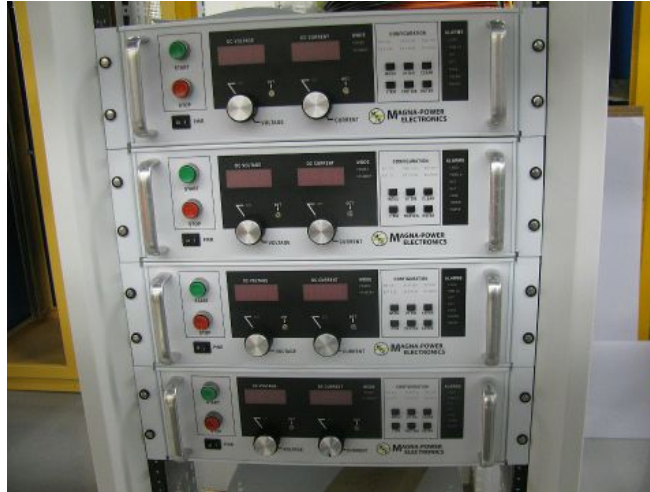
Figure 4.89. Example of a Switch Mode Power Supply.
