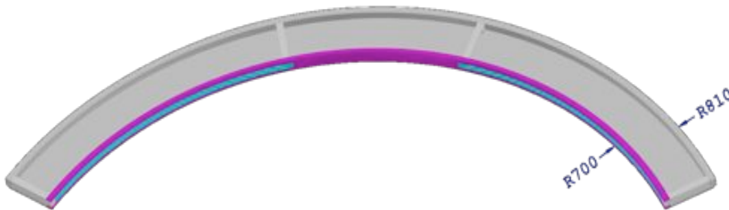
Figure 8.8. Panel without covers or straws. Magenta regions are stainless steel alloy 316; gray are aluminum; and cyan is plastic. Dimensions are in millimeters.
