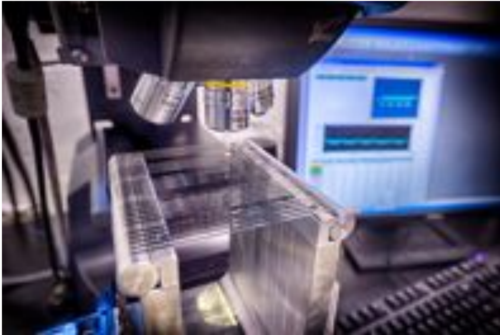
Figure 4.54. First stage prototype at the optical test stand. The stand provides surface elevation measurements along and across ribbons at sub-micron accuracy.
