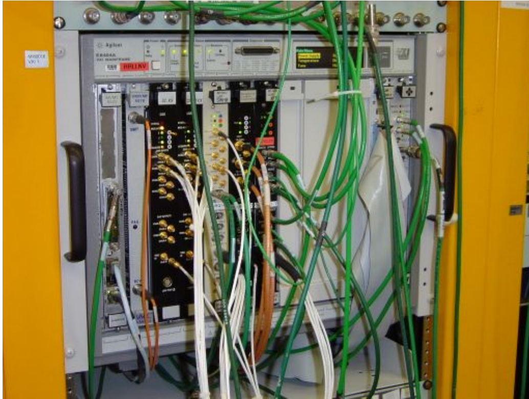
Figure 4.67. The Recycler LLRF system. Slot 0 is the controller. Slot 1 is the Reflective Memory. Slot 2 is the RF Switch (SWH). Slot 3 is the Direct Digital Synthesizer (DDS). Slot 4 and 5 is the Digital Signal Receiver (DSR). Slot 6 is the Transfer Synchronization (XFR). Slot 7 is the Direct Input/Output Module (IO 100). Slot 8 is the Multi-channel field controller (MFC).
