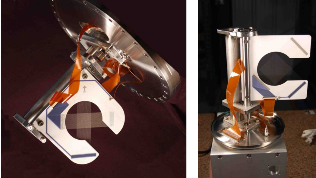
Figure 4.20. Slotted ceramic board holds both horizontal and vertical wire planes. The ceramic is slotted to allow it to be moved into and out of the beam path with beam present.
