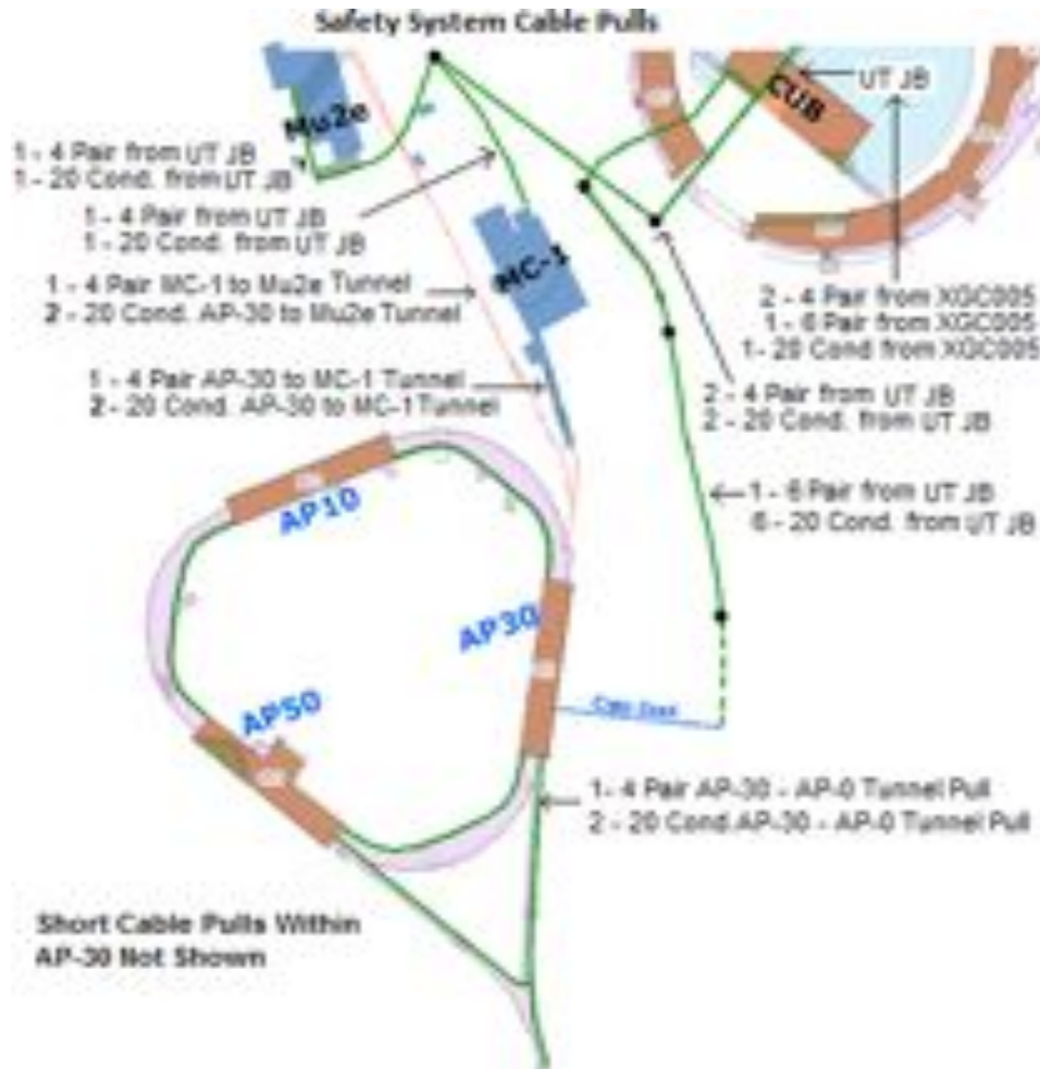
Figure 4.31. Safety System Interlock Cable pulls [50].
