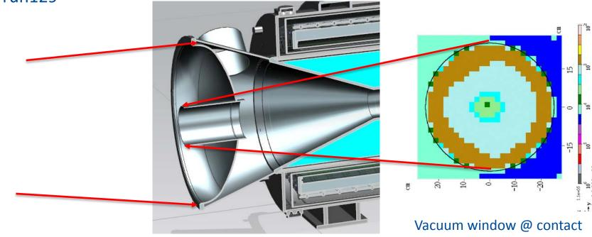
In situ end cap @ contact 32 rem/hr (321 mSv/hr) Vacuum window @ contact Separated from PS 1 to 7 rem/hr (10 to 70 mSv/hr)
