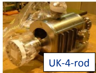
Compact cavities aiming at small footprint & 400 MHz , ~5 MV/cavity
