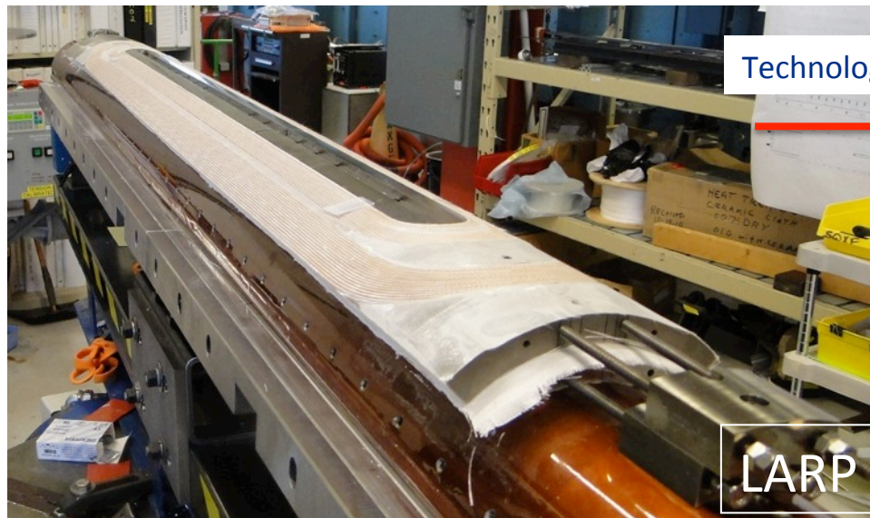
Winding with no "popped strands" in 40-strands Rutherford Cable
