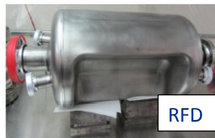
Compact cavities aiming at small footprint & 400 MHz , ~5 MV/cavity
