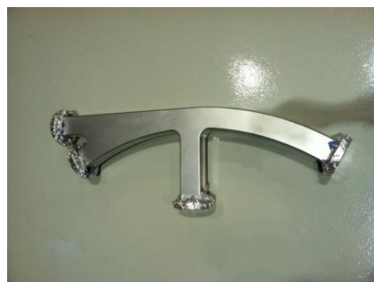
Vacuum chambers for dipoles (received)
