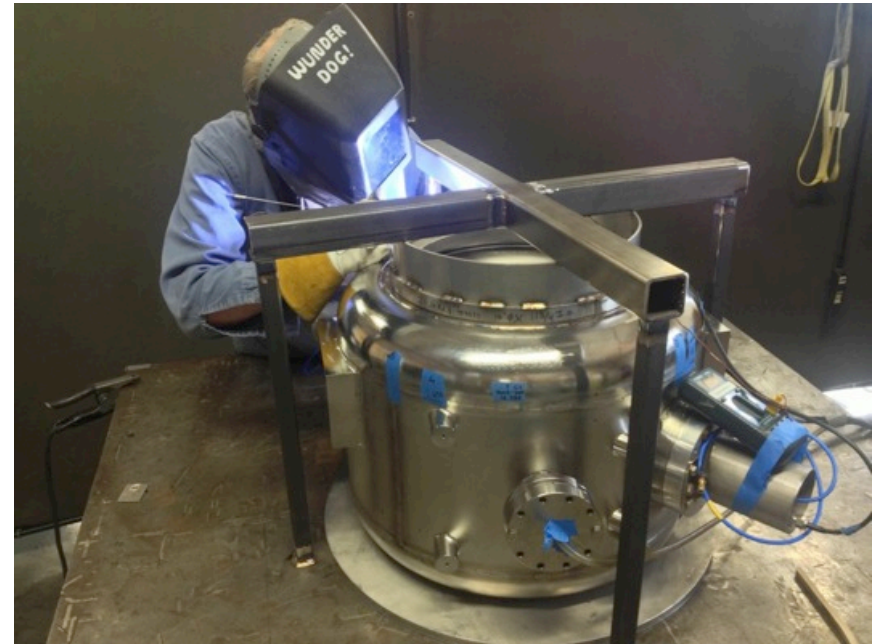
Large fixtures needed to control warping
