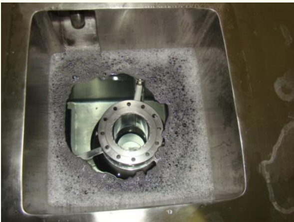
Cleaning of Single cell Niobium Cavity after EP
