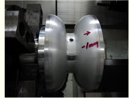
Machining of dumbbells on precision lathe
