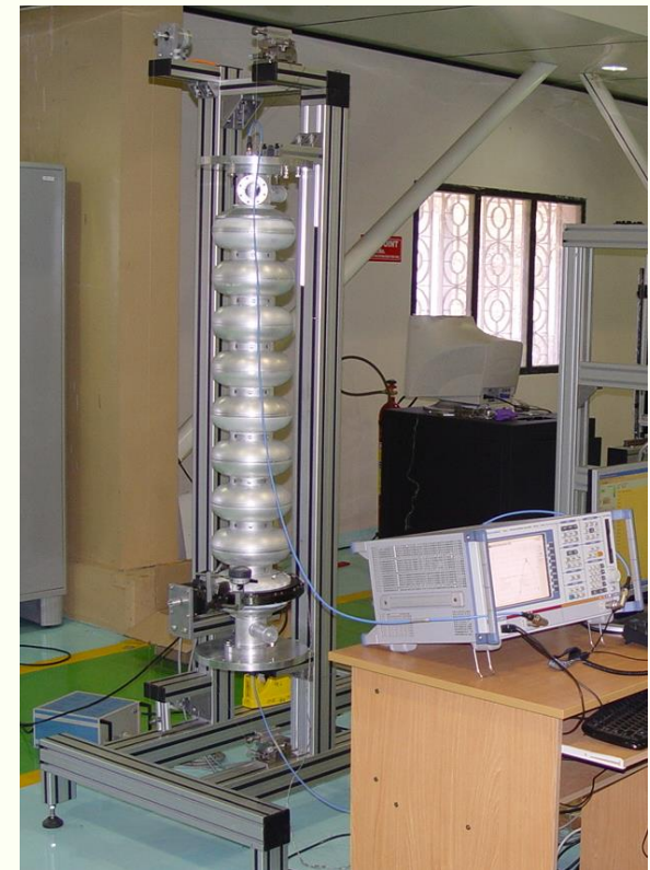
Manual Tuning of 1.3 GHz nine-cell cavity
