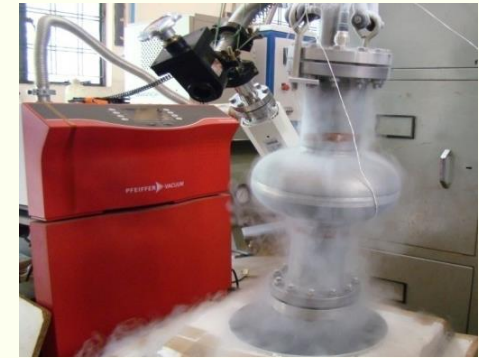
Leak testing at 77 K
