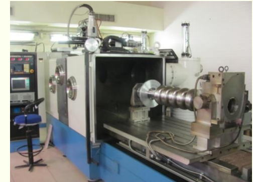
Final mid equator welding
