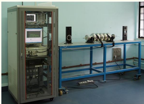
RF testing (Bead pull measurement)
