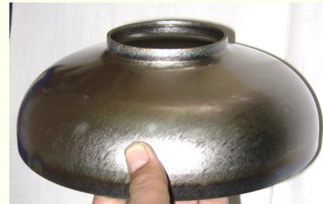
1 st formed niobium half-cell
