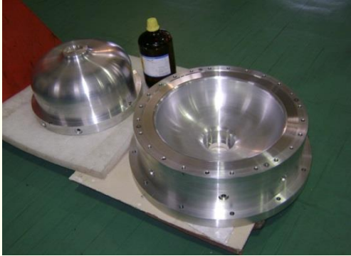
Half cell forming die & punch set
