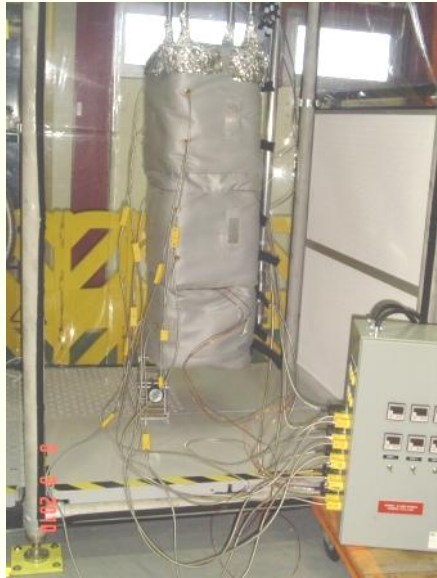
Low temp bake 120 C - 48 Hrs
