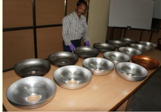
Formed Half cells (Aluminum, Copper, Niobium)
