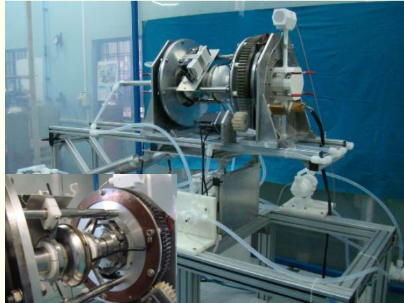
Electropolishing setup for 1.3 GHz and 650 MHz cavities
