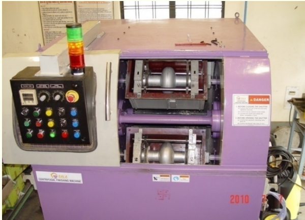
Barrel polishing machine for single-cell 1.3 GHz SCRF cavity
