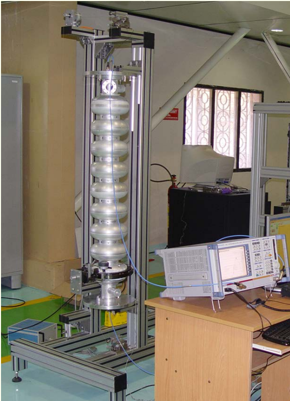
Tuning of 1.3 GHz nine-cell cavity
