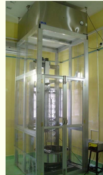
High Pressure Rinsing setup
