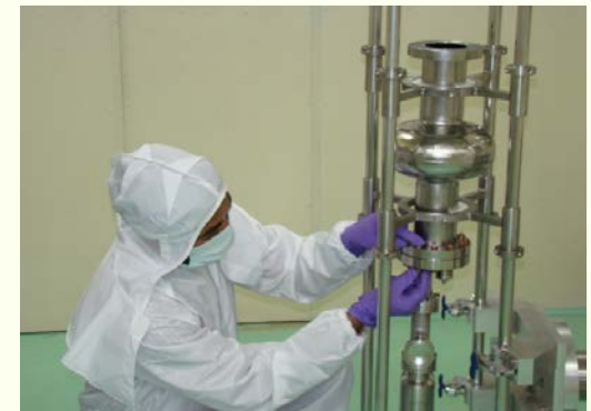
Preparation of cavity for VTS test in clean room
