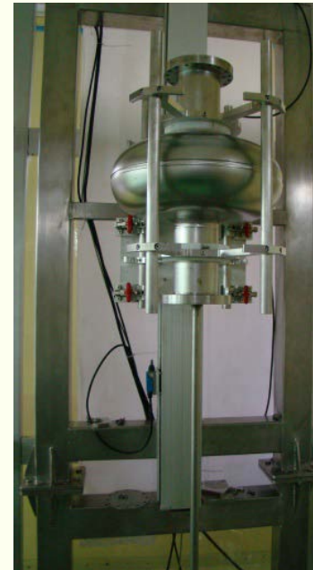
HPR of 650 MHz single-cell cavity
