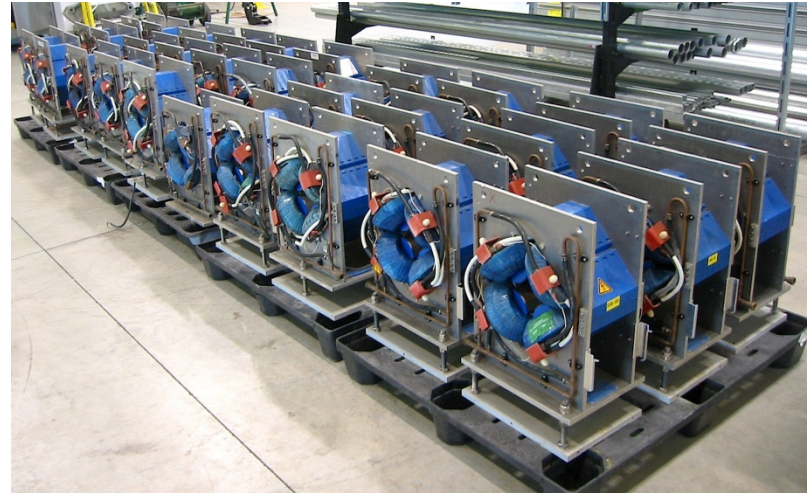
32 quads from JINR (Dubna) being measured
