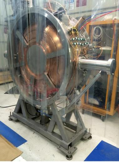
RF Cavity – Electro polished cavity body
