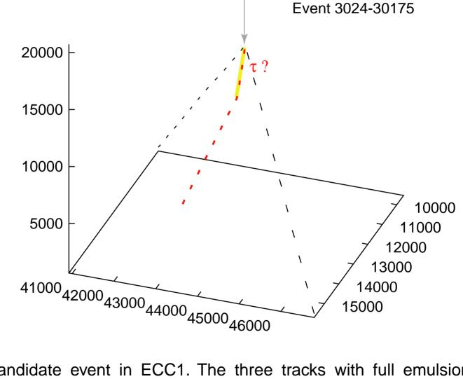
Candidate event in ECC1. The three tracks with full emulsion data are shown. The red track shows a 100 mrad kink 4.5mm from the interaction vertex. The scale units are microns.
