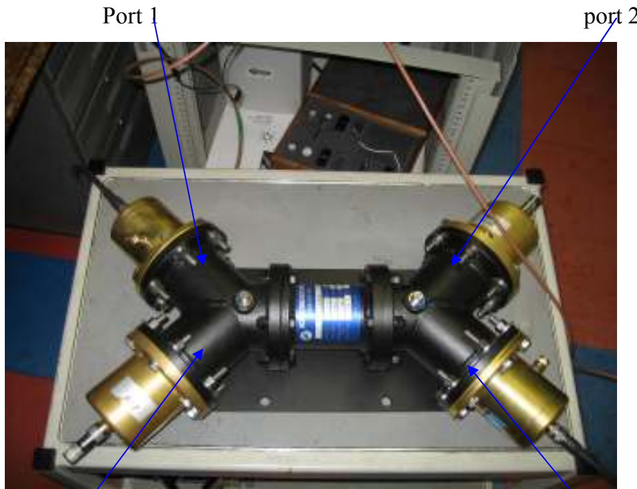
Fig. 6 400KW peak power quad hybrids
