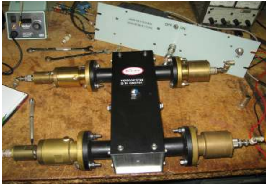
Fig. 3 the Dielectric Quadrature Hybrid with connectors
