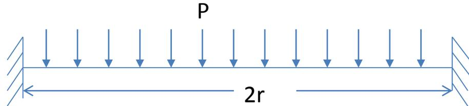
Max. Bending Moment at the outer rim of the clamped circular plate is:
