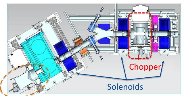
Scheme of PXIE IS and LEBT in final configuration
