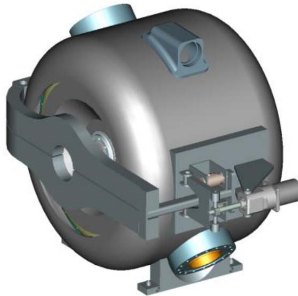
Figure 3.18: SSR1 cavity, helium vessel, and tuner.
