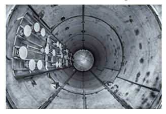
Several current and future neutrino experiments will use liquid-argon detectors, such as the MicroBooNE detector pictured here, to discover new physics. The LArSoft software package was created specifically for these experiments, including MicroBooNE and the future DUNE and SBND. *Photo: Reidar Hahn*
