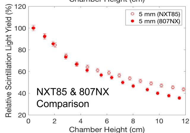
Absolute reflectivity measurements for NXT85 and 807NX PTFE materials are 97.5% and 96.1%, respectively<sup>[2]</sup>.
