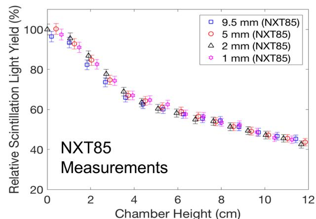
There is no dependence on the thickness of both PTFE materials for the reflectance of 178nm xenon scintillation light for the tested thicknesses in the range of 1 mm to 9.5 mm within uncertainties.
