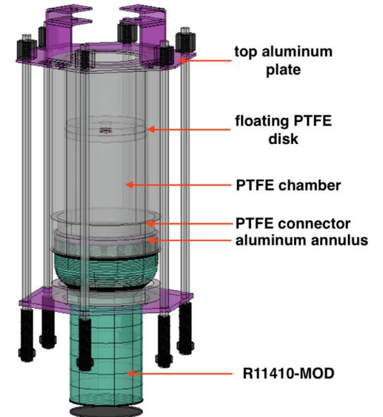
Mono-energetic scintillation light of 178 nm is generated by the 5.304 MeV  $\alpha$  particles emitted from a <sup>210</sup>Po source in the floater through ionization and excitation of xenon atoms.
