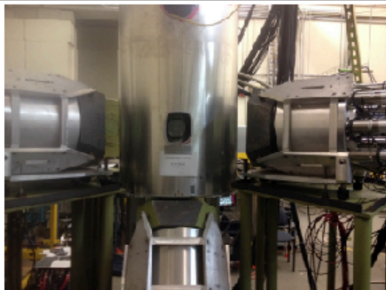
The Compton scattering setup at HIGS to measure proton's spin polarizabilities: Cryogenic target + NaI Array (HINDA)
