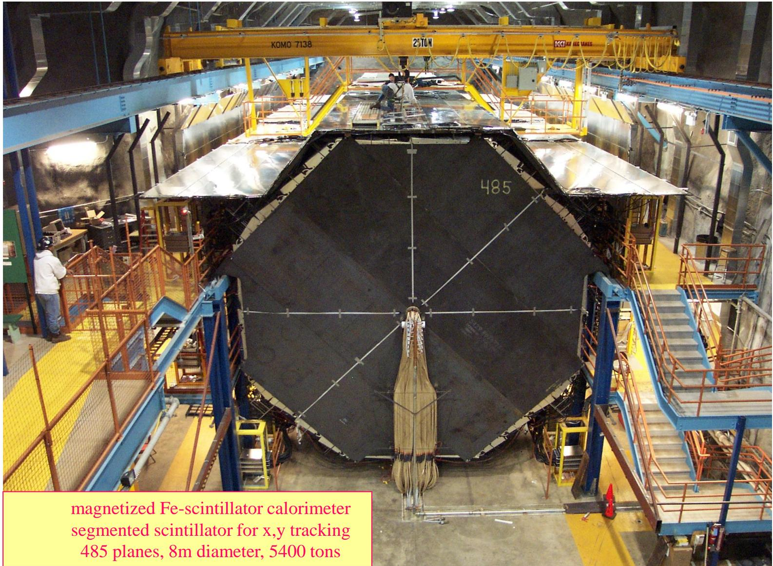
magnetized Fe-scintillator calorimeter
