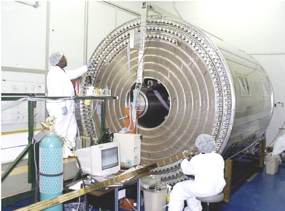
Figure 4. The COT during "stringing" of the wire planes and field sheets. The carbon composite inner cylinder, aluminum end plate (east) and aluminum outer cylinder are visible. Superlayers 1-5 have been strung and superlayer 6 is about half done. A wire plane is inserted at 10:00 and a field plane at 4:00. Pre-tension fixtures are seen in superlayers 6 - 8.
