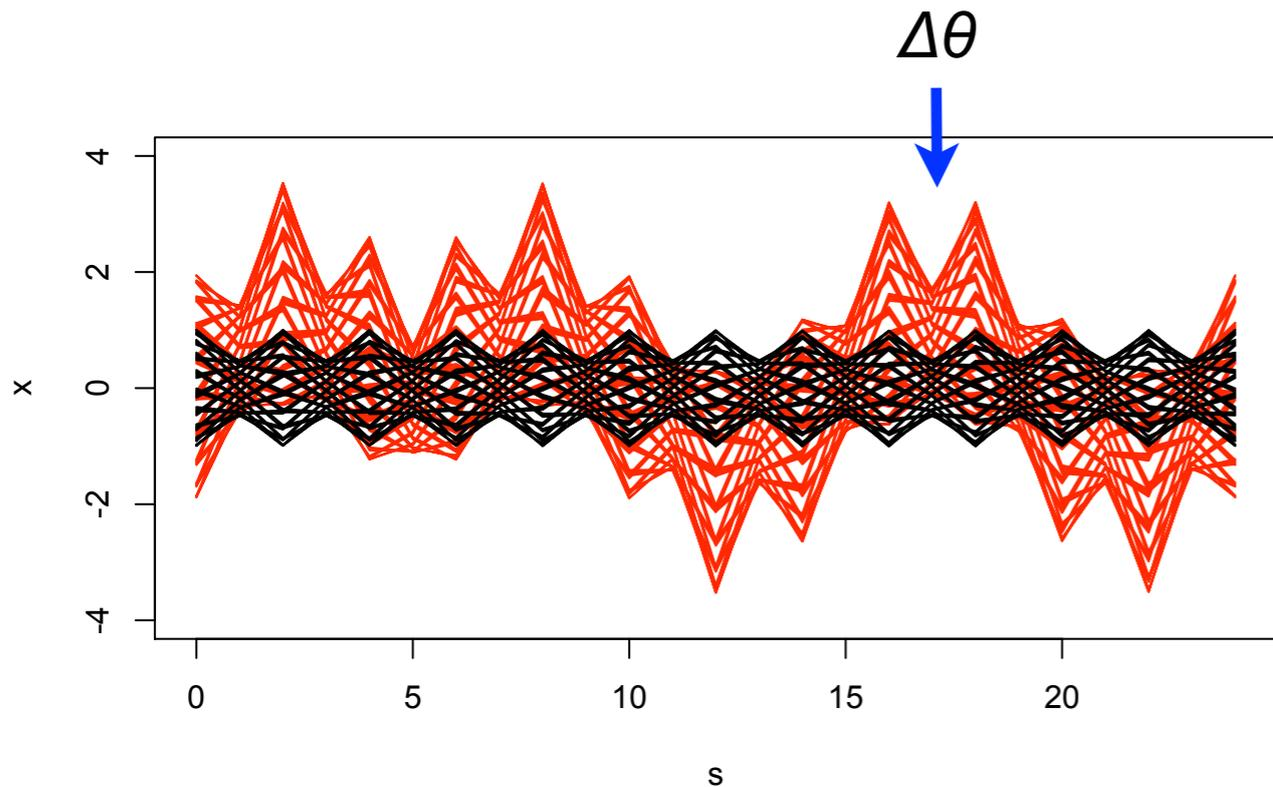
Orbit distortion due to single dipole field error
