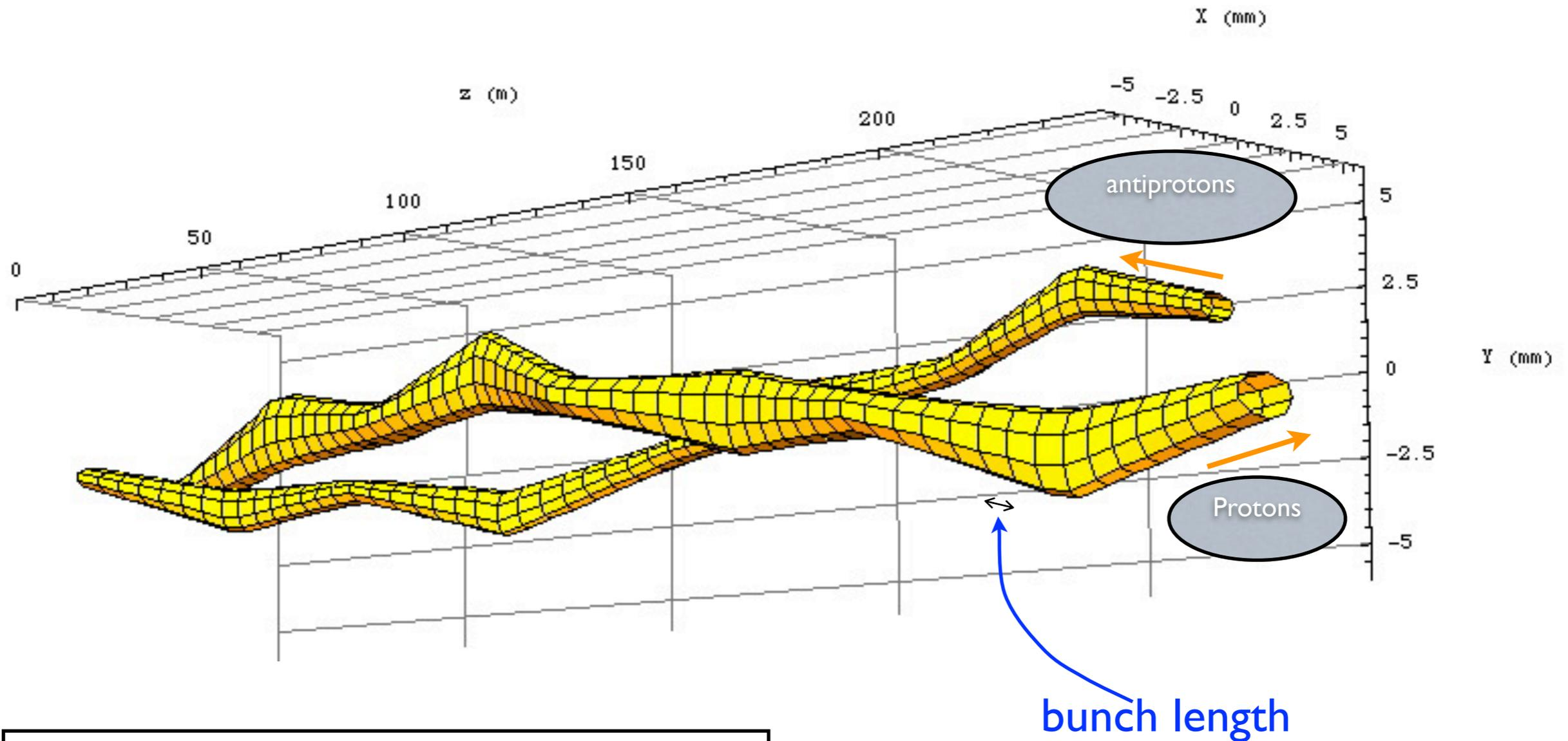
Helical orbits through 4 standard arc cells of the Tevatron
