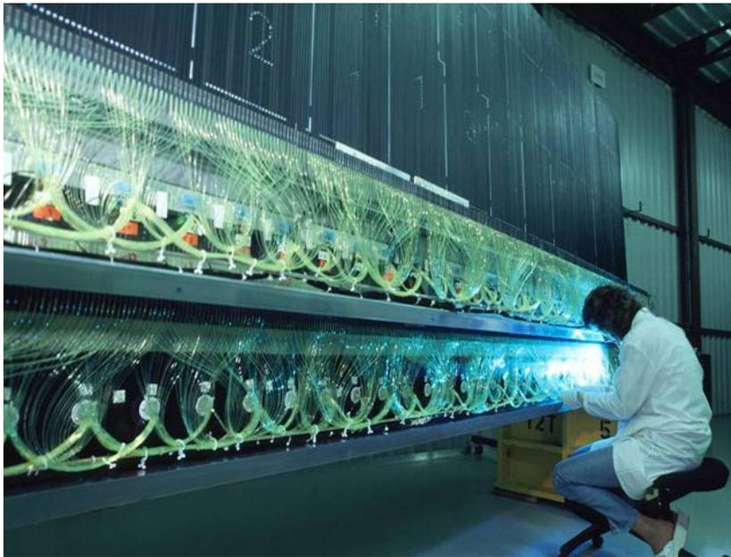
The iron structure supporting the calorimeter (girder) contains the return field of the ATLAS 2 Tesla solenoidal field. The photon-sensors are inside the girder and in a modest B-field
