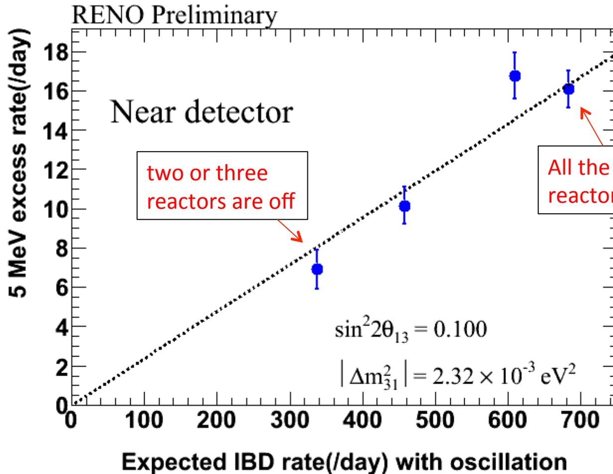
5 MeV excess has a clear correlation with reactor thermal power !
