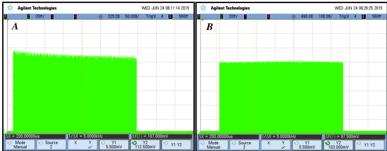
Figure 17. A) Pulse train oscilloscope output without timing adjustments, showing a negative slope. B) Pulse train oscilloscope output after pump diode timing adjustments were made, showing the desired flat pulse train for 2000 pulses per train.
