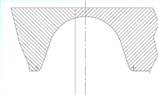
Nonsymmetrical mould for hydroforming
