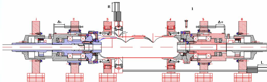
Principle of DESY necking equipment
