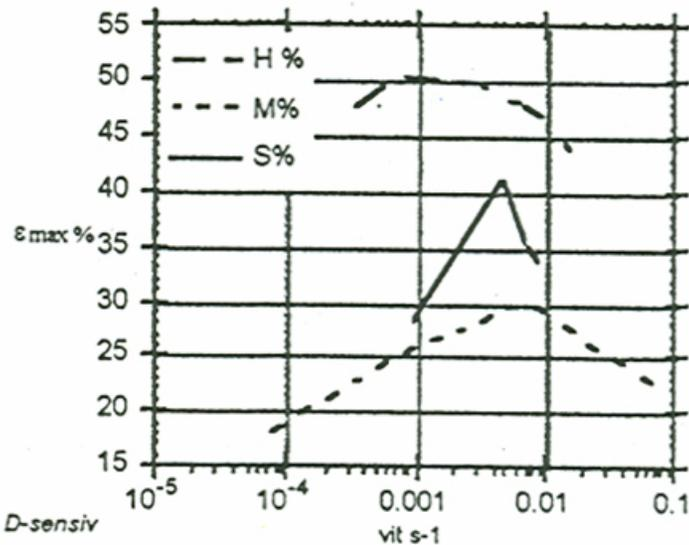
Dependence of maximum elongation of niobium versus strain rate (H, M, S different literature data).
