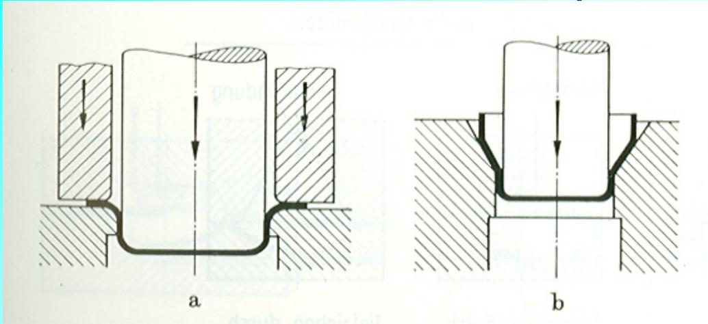
Principle of deep drawing; a-first step, b-second and further steps
