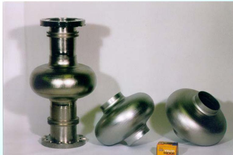
Fabrication of the seamless pot from Nb plate by spinning is possible without intermediate annealing
