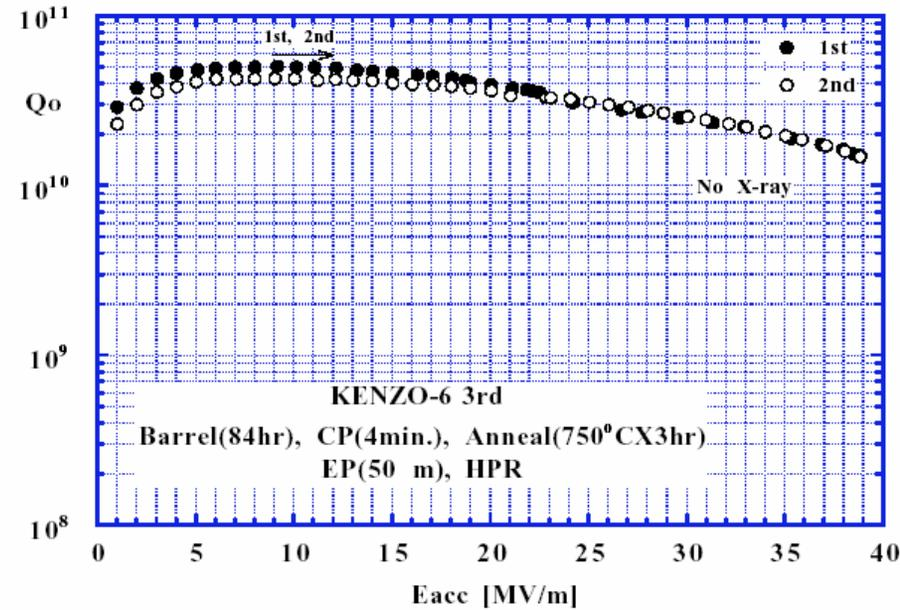
Some best seamless single cell cavities. Preparation and RF tests: K.Saito, P.Kneisel
