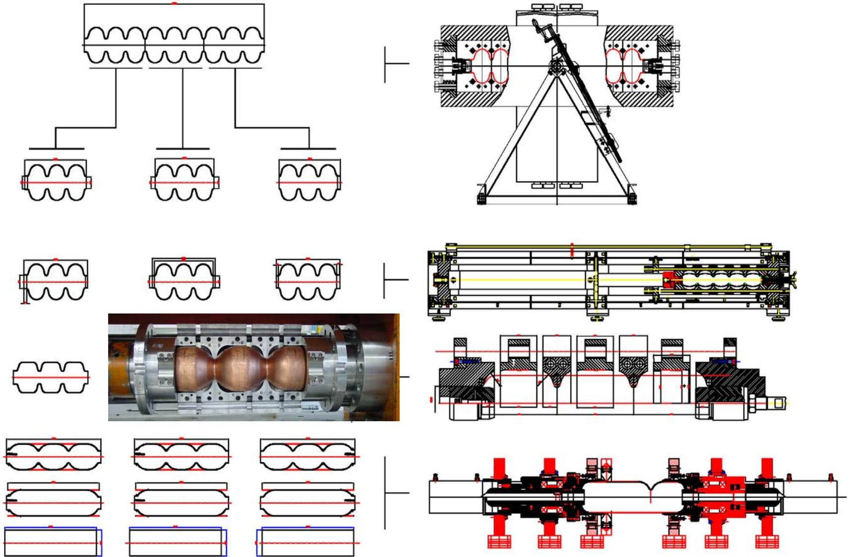
Z145: 9-cell as 3x3 cell cavity hydroformed at DESY, completed at E.ZANON (reached ca. 30 MV/m).
