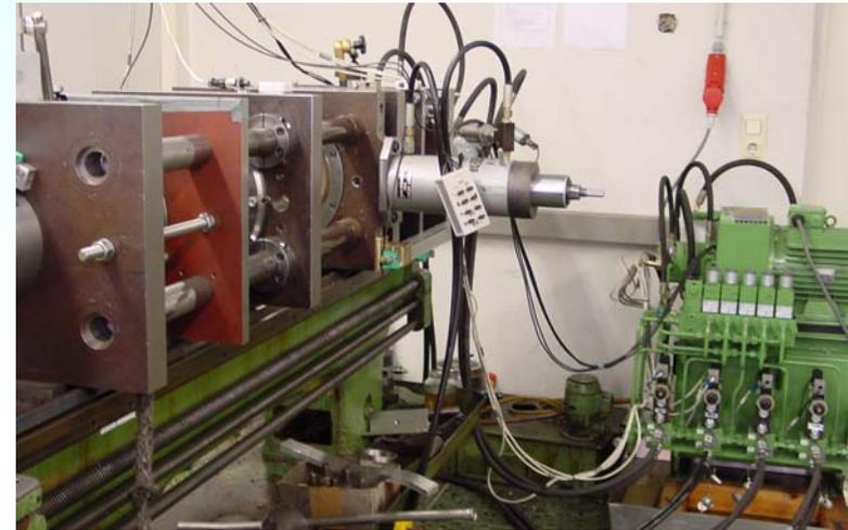
DESY Necking machine: new PC controlled necking procedure
