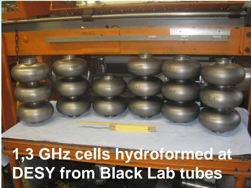
1,3 GHz cells hydroformed at DESY from Black Lab tubes
