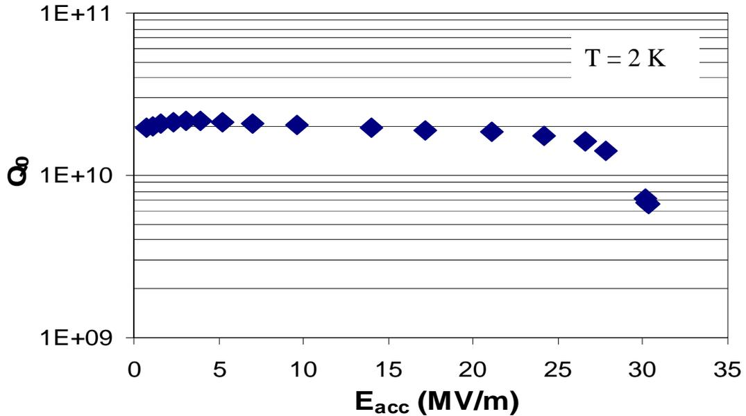
Surface treatment at DESY: 40  $\mu\text{m}$  BCP, 800  $^{\circ}\text{C}$  heat treatment, tuning; 170  $\mu\text{m}$  electropolishing (EP), ethanol rinsing, 800  $^{\circ}\text{C}$  heat treatment; 48  $\mu\text{m}$  EP, HPR, assembly and evacuation
