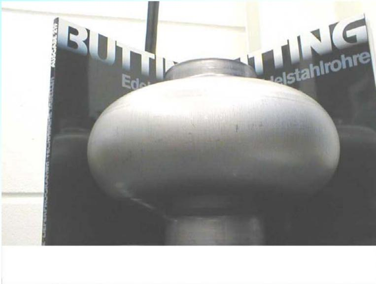
Single cell cavity fabricated at Fa. Butting (Germany) in collaboration with DESY from deep drawn tube produced at the company B.J. Enterprise (USA) (reached 39 MV/m)
