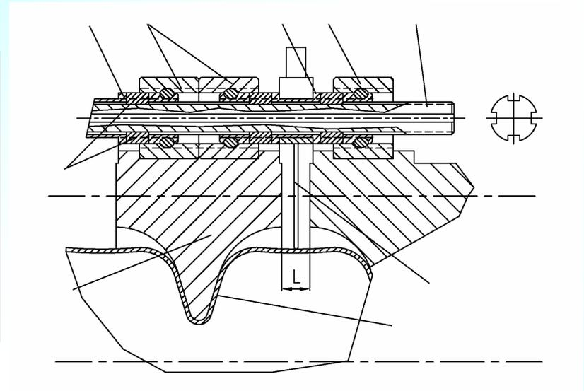
Synchronization mechanism for multi cell fabrication by hydroforming
