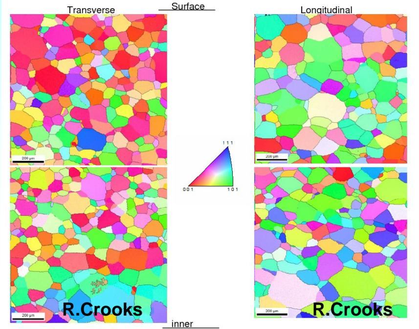
Microstructure and texture of Nb tubes produced by combination of spinning and flow forming
