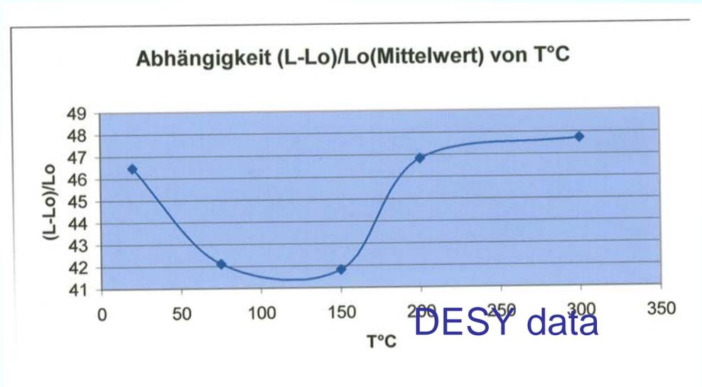
Dependence of the elongation on temperature. It make sense to perform hydroforming of niobium at room temperatures
