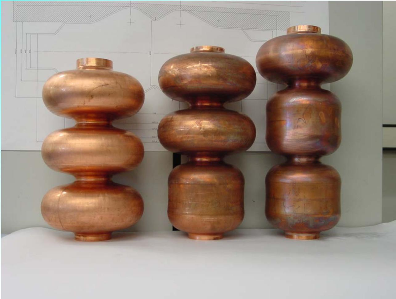
Hydroforming of cells can be done or as three cells simultaneously or cell by cell (hydroforming of the 9-cells from one tube piece can be done on the same way)
