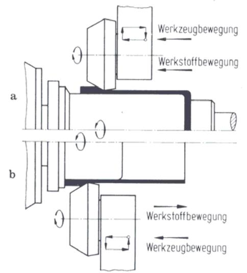
Flow forming of niobium spun tubes at MSR (Germany). Precise wall thickness after flow forming. Tolerances within of  $\pm 0,1$  mm
