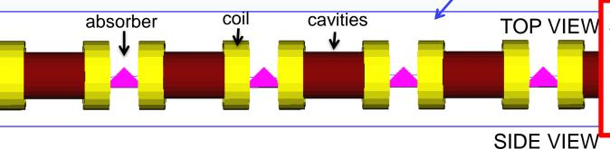
Tapered channel: The focusing field becomes progressively stronger to reduce the equilibrium emittance.
