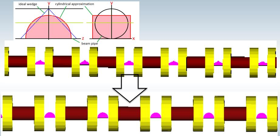
Replace liquid hydrogen (LH) absorber wedges with cylindrical absorbers.
