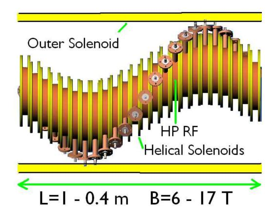
Guggenheim Vacuum rf Helical Cooling Channel High pressure gas rf
