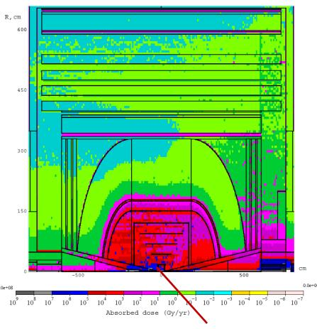
~1 MGy/yr for 2 beams, Comparable to LHC
