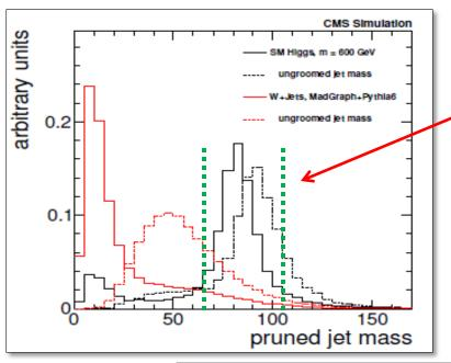
**Grooming techniques**: remove soft radiation and pileup from the jet (e.g., pruning)
