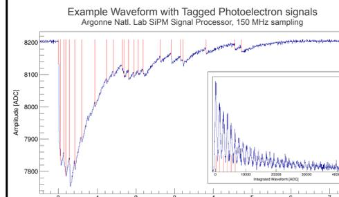
With the fast response of the SiPMs and the high-resolution sampling of the custom data acquisition electronics built by Argonne National Lab, fine details in the time structure of the scintillation signal are easily resolved. The SiPM response to photoelectrons is linear, meaning the signal strength can be easily converted into a measure of detected photons.
