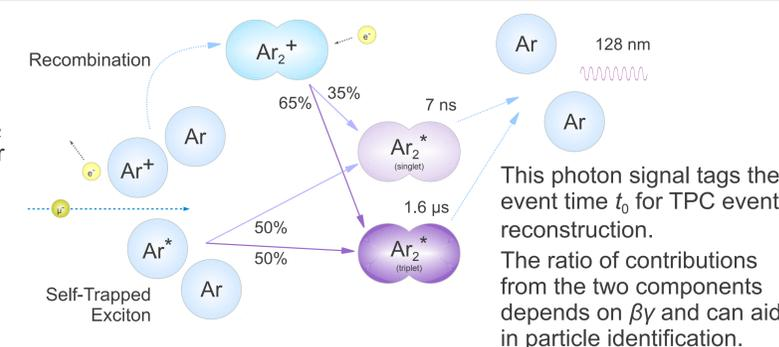
This photon signal tags the event time  $t_0$  for TPC event reconstruction. The ratio of contributions from the two components depends on  $\beta\gamma$  and can aid in particle identification.
