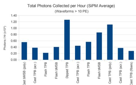
Results from the October 2013 TallBo visit identified the preferred quantity of waveshifter for the flash-heating method. The most promising designs to emerge from the March 2014 tests were acrylic dip-coated with TPB and polystyrene cast with TPB (above). In each run, relative performance in the free run data agrees with observations from hodoscope-triggered tracks.
