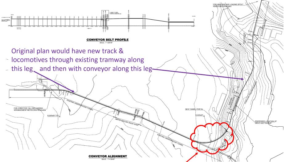
A single conveyor can be used if a new ~600' long tunnel and portal is excavated.
