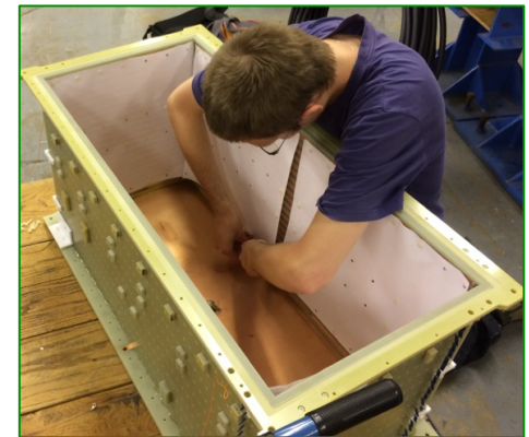
Test-mount of mock foil masks onto LArLAT TPC
