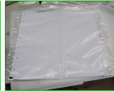
Reflector foil before/after TPB evaporation
