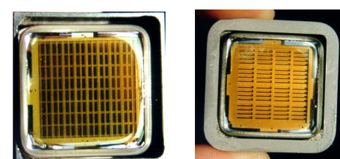
Two photographs of PMT detectors are shown side-by-side. The left one is labeled M64 and the right one is labeled M16. Both show a grid of scintillator strips within a metal housing.
