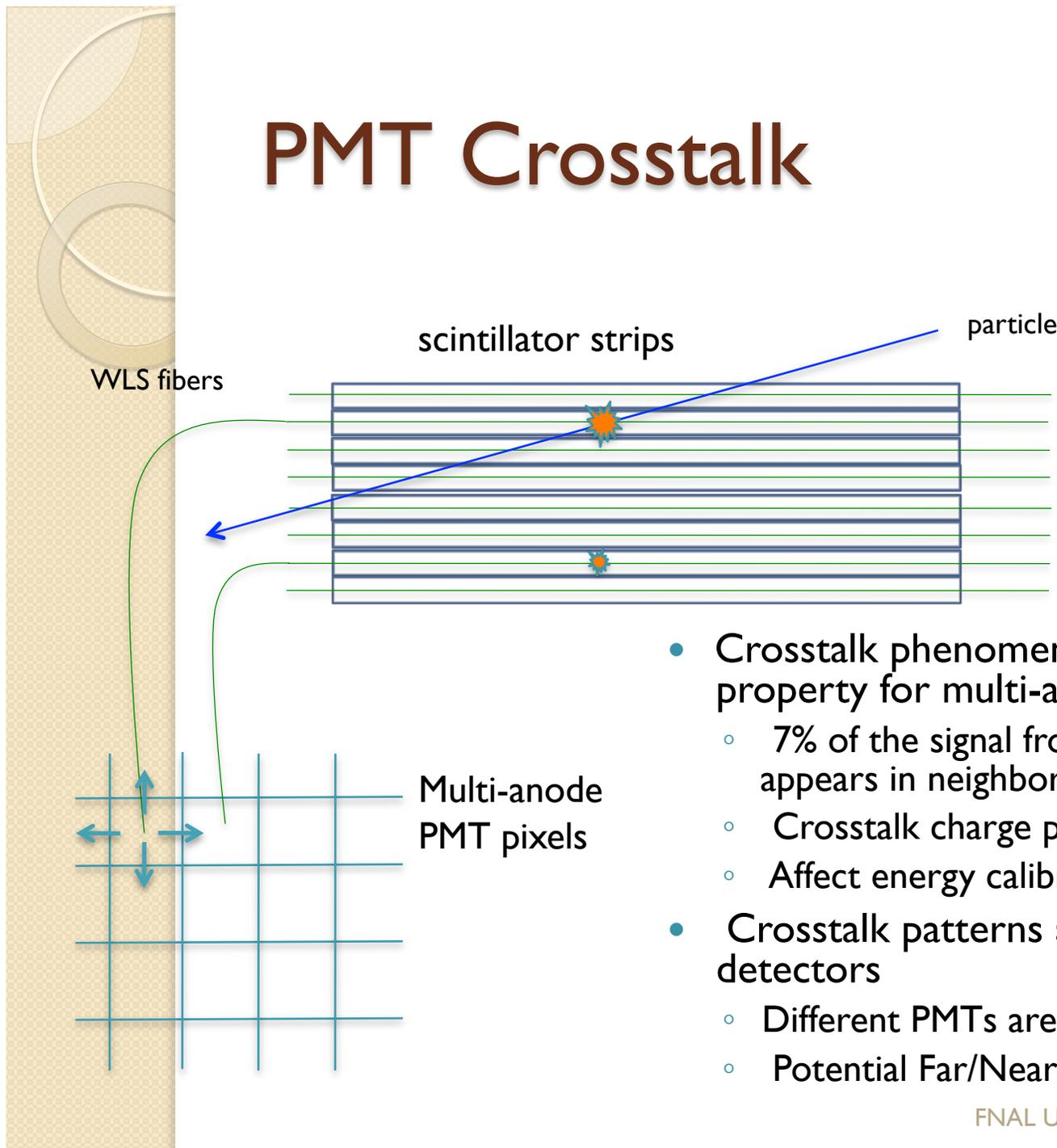
The diagram illustrates the PMT crosstalk phenomenon. It shows a stack of horizontal scintillator strips. A blue line representing a particle enters from the right and passes through the strips. Two interaction points are marked with starburst symbols. Green lines represent WLS fibers that collect light from the strips. On the left, a grid of multi-anode PMT pixels is shown with blue arrows indicating light signal transfer between adjacent pixels, representing crosstalk.
