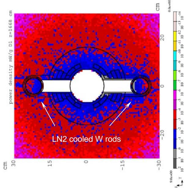
MARS model and power density (mW/g) in B1 dipole for case (ii) from two beams dumped after 1000 turns
