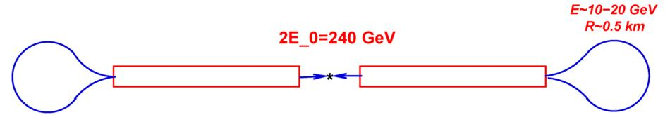
If  $\eta$  is the energy acceptance of the ring, the maximum energy of beamstrahlung photons should be  $\eta E$  (not  $\eta E_0$ ). This reduce L by a factor of  $(E/E_0)^{2/3} \sim 0.25$ . However, due to much lower SR losses  $(E^4/R)$  one can increase Nf by a very large factor and thus to increase the luminosity by 1-2 orders of magnitude (>10<sup>35</sup>).
