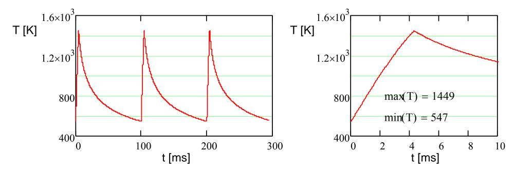
Dependence of maximum foil temperature on time, only radiative cooling is taken into account
