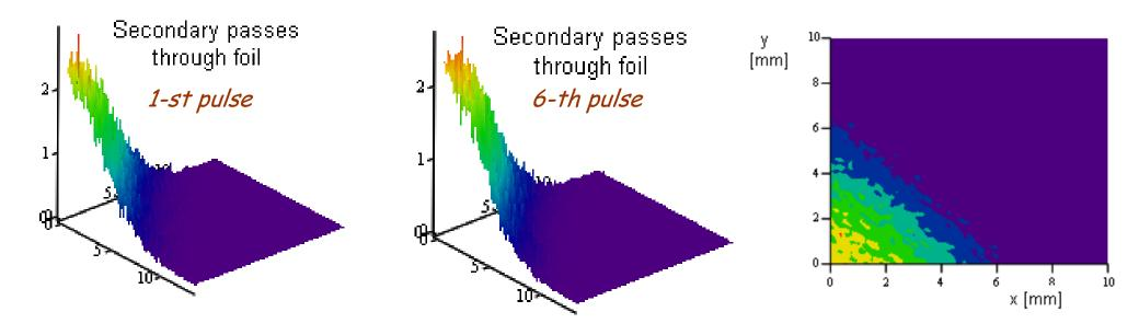
Density of particle passes through foil (mm<sup>-2</sup> per particle of single pulse)
