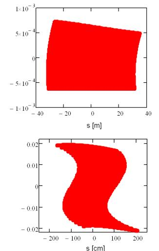
Longitudinal phase space at the end of injection and after compression
