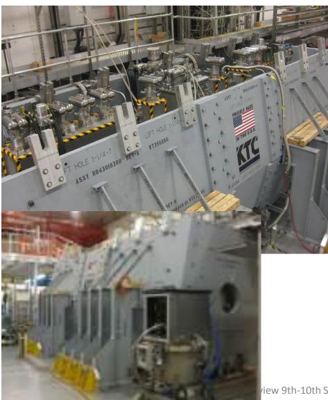
Flux return path to protect sensitive equipment from fringe field of magnet chain.
