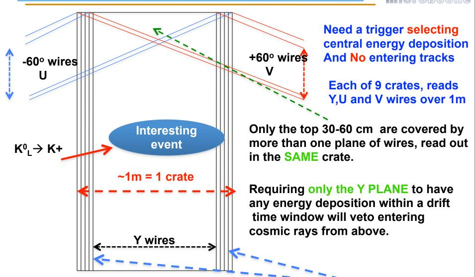
CR entering from sides: veto on energy deposition in L or R wires
